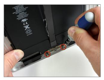
Remove the two 2.84 mm Torx screws securing the dock connector cable to the rear case.
